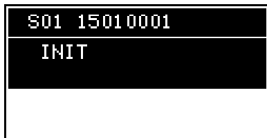
Fig. 3-18 Display during the start phase
